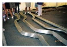
the finished rectangular profile with accompanying depressions and stiffening groves. This is done in a die that shapes the tube when the high pressure is injected into the capped tube.
