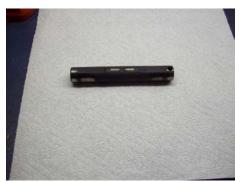
minimal wear evident. In the design of the C-2 suspension, the half shafts are the upper suspension link and the side yolks rest against the spider gear shaft and the weight of the car is pushing in against them. In normal
