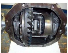
operation the yolks and the differential rotate together. Only if one tire is spinning or a small tire is installed on one side at the rear, or the car is in a turn would the yolk be spinning against the shaft. The slight radial grooving at the ends of the side yolks was removed holding the yolks
