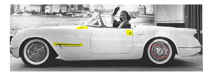
We do know that the Motorama wheel cover with the 90 degree flipper was placed into production but we do not know when it stopped. Russ Howay has car #68 and it has the 90 degree flippers so likely sometime after car 68 the wheel cover changed.
