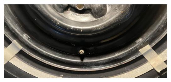
Note that with a 1953 through fall of 1954 style wheel cover, the grippers do hit the newly created nubs for the 1955 wheel.
