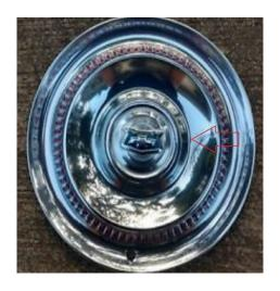
There are experts that will indent these wheel covers to make a 90 degree flipper or to make the more traditional wheel cover with the flippers in line with the Chevrolet Bowtie. However, they are different from the originals as the originals have indented on the rim the words "PAT PEND", PATENTED", "LYON" (the manufacturer) and "WHEEL COVER". The GM replacements do not have these marks.
