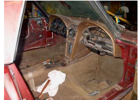
Note the AC ducts on this Big Block Mid Year.
