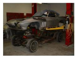
how bad the frame was until he had the body off the car. At that point, he discovered the inside frame rails were also rusted and much time was spent getting the frame right before dipping and
